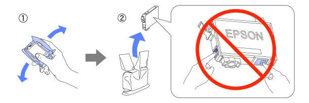
For the initial setup, make sure you use the ink cartridges that came with this printer. These cartridges cannot be saved for later use. The initial ink cartridges will be partly used to charge the print head. These cartridges may print fewer pages compared to subsequent ink cartridges.
