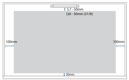
When you want to use the installed Touch Unit as it is, leave a gap of 25 to 100 mm between the bottom of the touch unit and the top of the image. If there is not enough space, you need to reinstall the Touch Unit.
