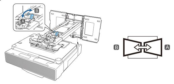
Turn the adjustment dial ③ in the installation guide to adjust the vertical tilt
