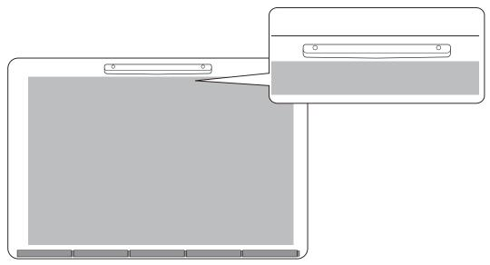
• If you are using a Touch Unit Bracket, make sure that the bottom edge of the bracket is flush with the edge of the projection surface without any gaps.
