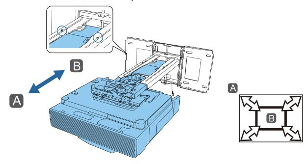
Loosen the M6 bolt, and then adjust the vertical slide
