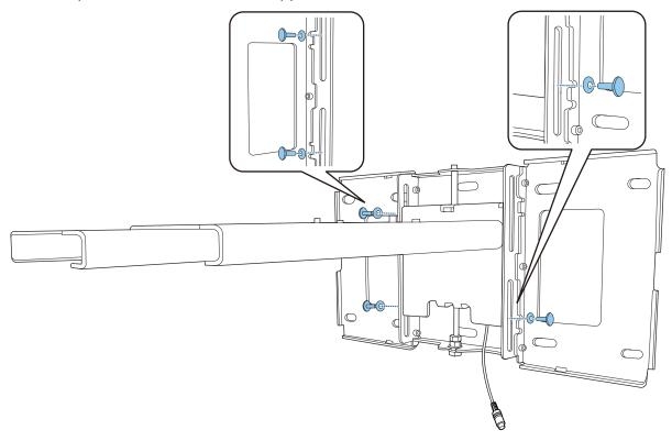
Adjust the vertical slide with the open-ended spanner to align the marks on the wall plate and the setting plate.
