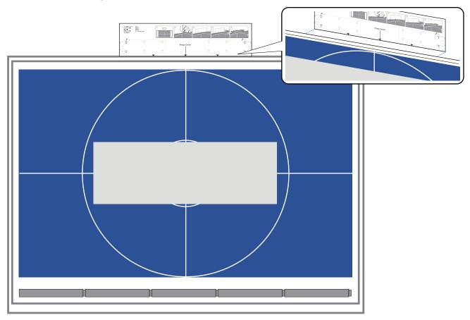
Drill holes in the installation surface, and then remove the template sheet Make holes at the four points labeled as **Main** on the template sheet.
