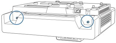
Loosen the M4 bolt on the adjustment unit, and then align the marks for each part
