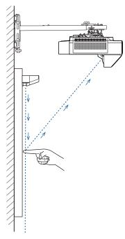
If the laser is not emitted parallel to the screen, the projector will not detect touch operations or the position of your finger correctly.
