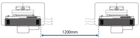
If you cannot secure a gap of approx. 1,200 mm, install a partition to block the heat vented from the projector's air exhaust vent.
