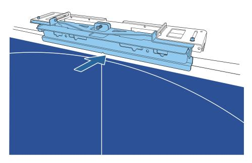
Slide it in until the lower edge of the bracket touches the projection screen.
