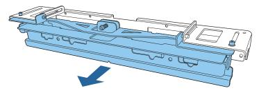
To prevent the sliding section from slipping during installation, lightly tighten the top screws (x2) that you loosened in step 6.
