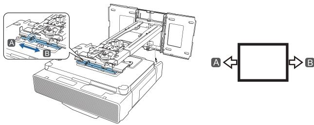
Loosen the M4 bolts (x2), and then adjust the forward/backward slide
