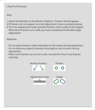
Turn the adjustment screw clockwise to cover the left and right pointers
