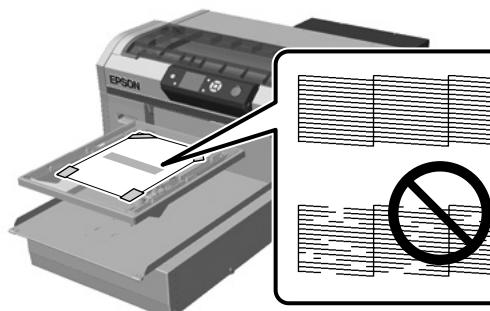
If there are no parts missing from the check pattern, attach the frame to the platen. If there are parts missing from the check pattern, see the *User's Guide* (Online Manual) - "Cleaning the print head" for information on cleaning the print head.
