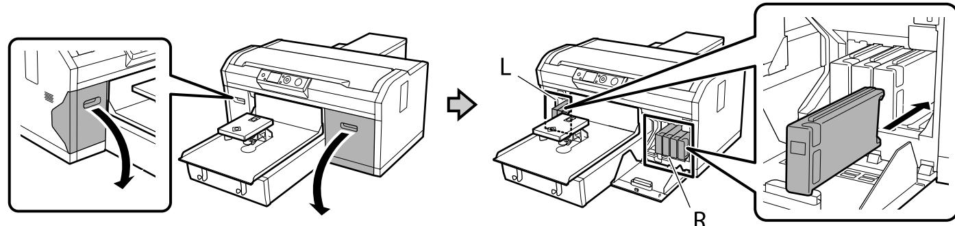
The ink colors you need to install vary as shown below depending on the Color Mode you will set. After making settings, you cannot change from High-speed Color Mode to another mode, or from White Ink Mode/Color Ink Mode to High-speed Color Mode.
