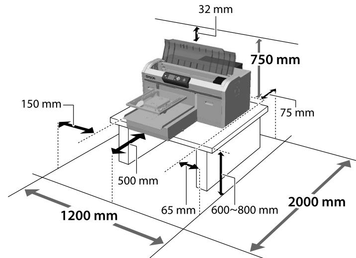
Install the printer on a stand and so on. Use a location that meets the following conditions.
