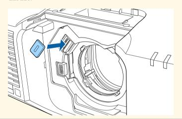
Insert the lens straight into the projector's lens socket with the white dot facing up.
