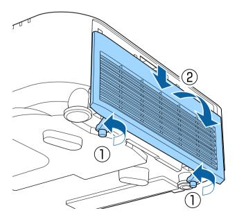
Pull the air filter out of the projector.
