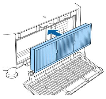
Replace the air filter cover as shown and tighten the screws.
