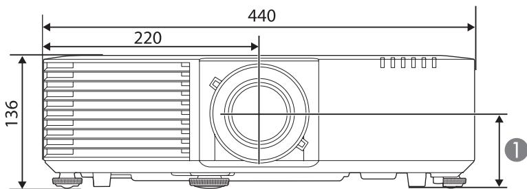
① Distance from center of lens to suspension bracket fixing point : 74 mm
