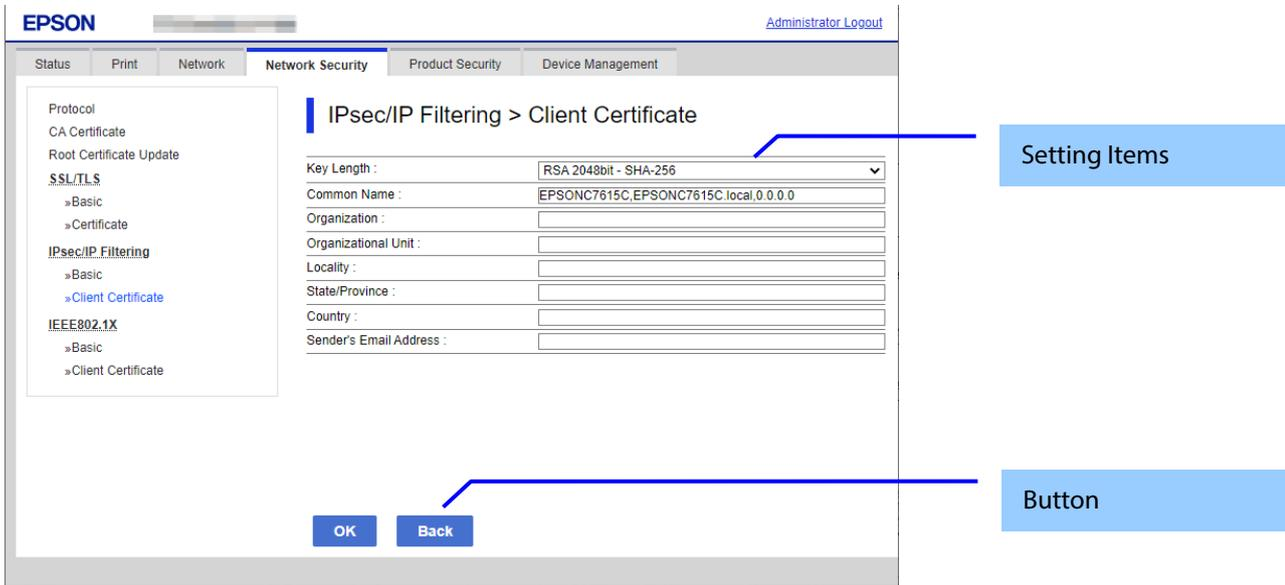
**Figure 10-52 Generate CSR(Certificate Signing Request)**
