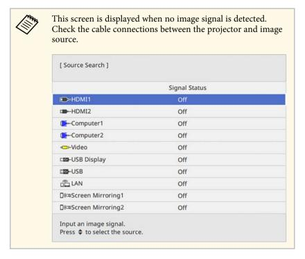
• Press the button for the source you want on the remote control. If there is more than one port for that source, press the button again to cycle through the sources.
