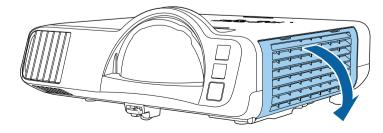
Pull the air filter out of the projector.
