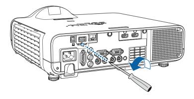
Connect the wireless LAN module to the USB-A port.
