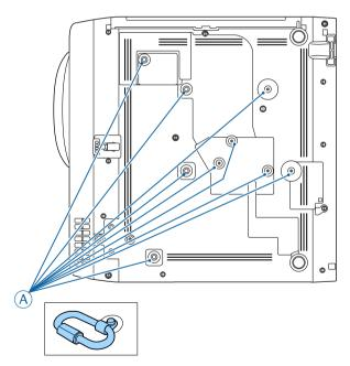
Attach the safety wire to a structure that is strong enough to bear the projector's weight, such as mounting hardware.
