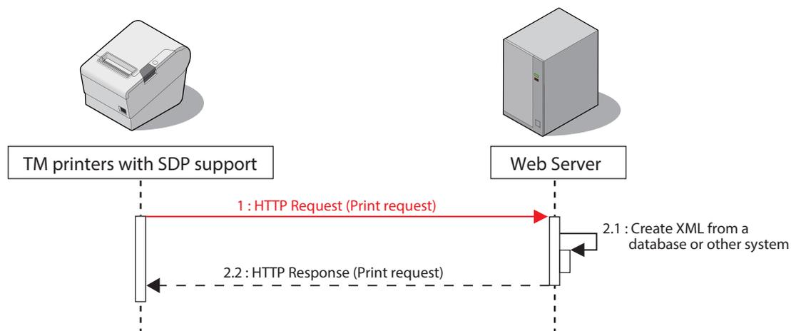
A TM printer with SDP support periodically sends a HTTP POST request (print request) shown below. The format of request message is URL-encoded form data (application/x-www-form-urlencoded). Set the sending destination and sending interval according to "Server Direct Print Settings" (page 28). If communication fails, it is attempted again after a specified interval.
