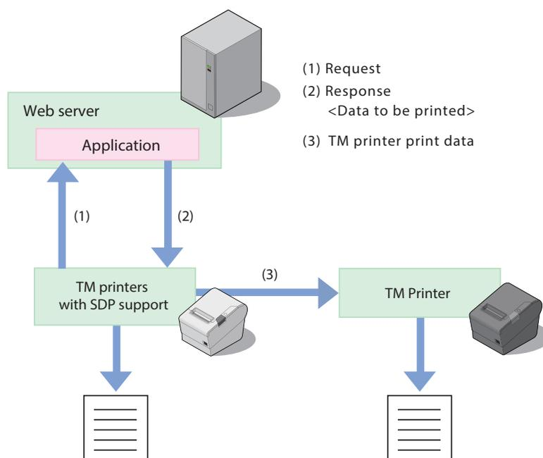
A TM printer with SDP support periodically sends a print request ((1) in the figure above) to the Web server. The Web server application includes print data in the response ((2) in the figure above) to a print request from the TM printers with SDP support. (When no print data exists, the Web server returns an empty response.) If print data for the TM printer is included in a response, the TM printers with SDP support controls the TM printer in order to do the printing ((3) in the figure above).
