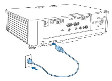
The projector's power indicator turns blue. This indicates that the projector is receiving power, but is not yet turned on (it is in standby mode).
