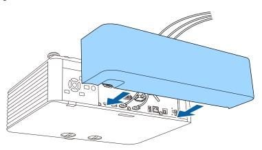
**3** Tighten the cable cover screws.
