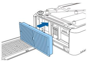
• Close the air filter cover and tighten the screws.
