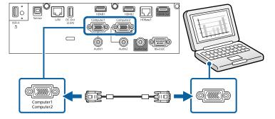
**3** Tighten the screws on the VGA connector.
