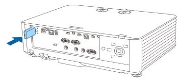
Attach the cover comes with your wireless LAN module, and secure it in place with the screw.
