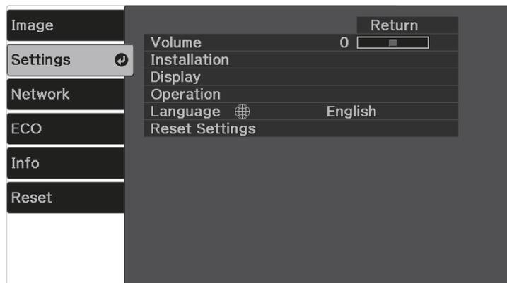
**4** Select **Installation > Pattern > Test Pattern**, and press [Enter].
