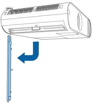
4 Pull the air filter out of the projector.
