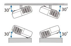
If you use the projector tilted at an angle of more than  $30^{\circ}$  it could be damaged and cause an accident.
