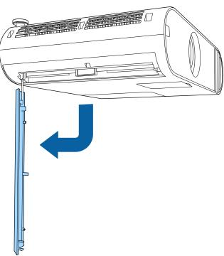
**3** Pull the air filter out of the projector.
