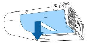
Loosen the screws securing the lamp to the projector. The screws do not come all the way out.
