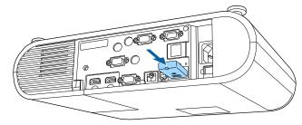
Attach the wireless LAN module cover, and secure it in place with the screw.
