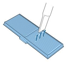
Place the air filter so that the runners on both sides of the filter follow the guide grooves on the projector, and push it up gently until it is in a position from which it does not fall down.
