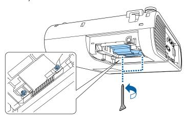
**6** Grip the raised section of the lamp and remove it.
