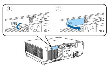
**3** Connect the Wireless LAN module to the wireless LAN module slot.
