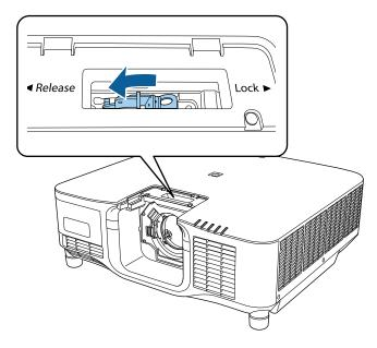
Insert the lens straight into the projector's lens socket with the white dot facing up.
