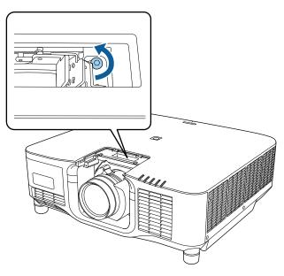
Hold the lens firmly as you pinch the lock lever and move it to the **Release** position.
