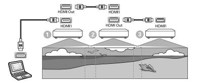
Connect the projector to the computer using the HDMI cable, and then connect the HDMI1 In port and HDMI Out port of the projectors using the HDMI cable.
