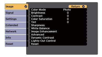
Press the up or down arrow buttons to move through the menus listed on the left. The settings for each menu are displayed on the right.
