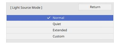
If you set the **Light Source Mode** setting to **Custom**, select **Brightness Level** and use the left and right arrow buttons to select the brightness.
