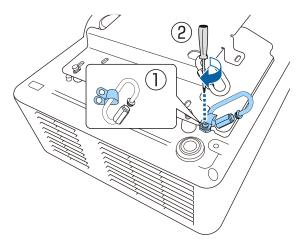
Loop the safety wire through the carabiner on the ceiling mount, and attach both ends to the carabiner on the projector.
