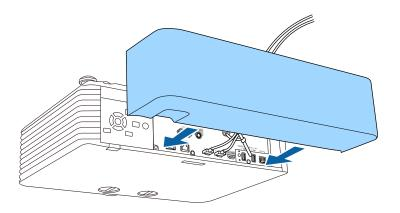
**3** Tighten the cable cover screws.
