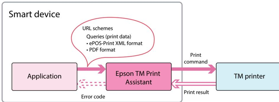
An application invokes Epson TM Print Assistant by the URL scheme and uses queries to transfer print data to it. When Epson TM Print Assistant receives print data, it sends a print command to the TM printer. The TM printer returns the print result to Epson TM Print Assistant. When the print result is an error, Epson TM Print Assistant displays an error message according to received status.
