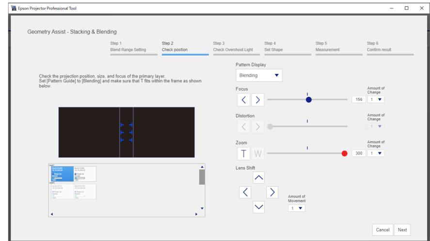
If you select **Flat** as the **Projection Screen Type**, T-shapes are displayed on the projection surface. See the following examples to adjust the projection position and size.
