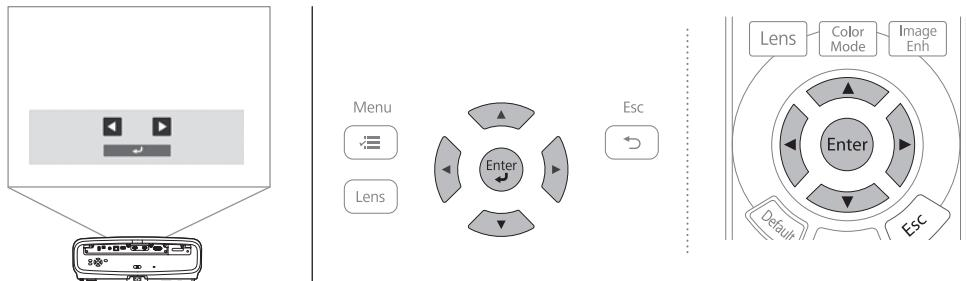
**EN** The first time you turn on the projector, the setup wizard is displayed. Make the focus, projection direction, and language settings using the arrow and [Enter] buttons on the control panel or remote control.
