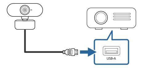
Connect a commercially available webcam with a microphone to the USB-A port of your Google TV projector. (You do not need to connect a webcam with a microphone to launch this app.)
