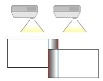
• Select the **Blend Curve** setting and select a gradient for the shaded area on the projectors.
