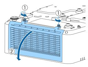
Pull the air filter out of the projector.
