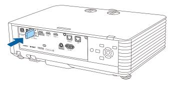
Attach the cover comes with your wireless LAN module, and secure it in place with the screw.
