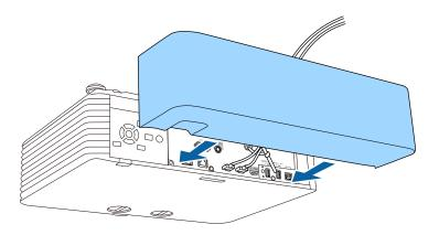
**3** Tighten the cable cover screws.
