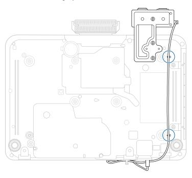
After connecting the end of the USB cable to the projector, loop the cable tie through the cable holder of the projector, and then fold the USB cable and fix with the cable tie.
