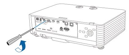
**2** Connect the wireless LAN module to the USB-A port.
