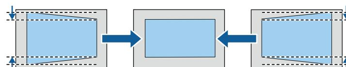
If you have adjusted the position of the projected image by using the lens shift feature, adjust the V-Balance and H-Balance settings as necessary.
