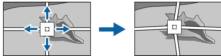
**10** If you want to correct all points in a specified vertical column or horizontal row at once, hold down the [Enter] button for two seconds.
