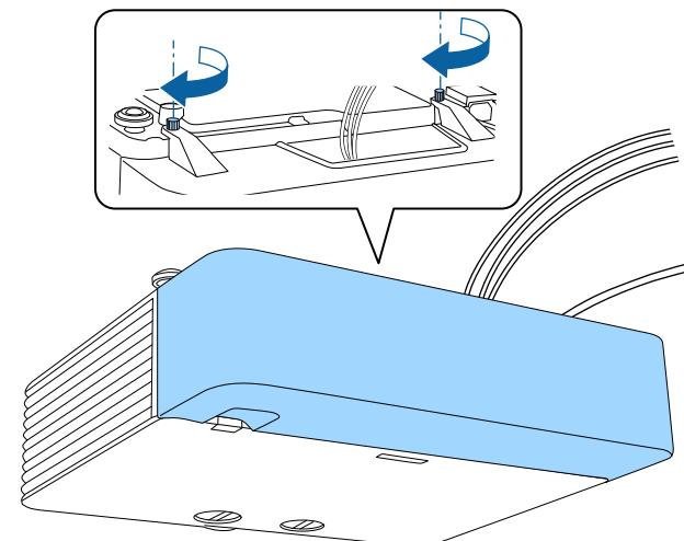
To remove the cover, loosen the cover screws and pull the cover off of the projector.
