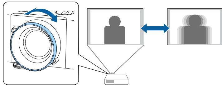
You can correct the focus using the center focus ring and corner focus ring. (EB-L790SE/EB-L795SE/EB-L690SE/EB-L695SE/EB-L790SU/EB-L690SU/EB-L695SU)
