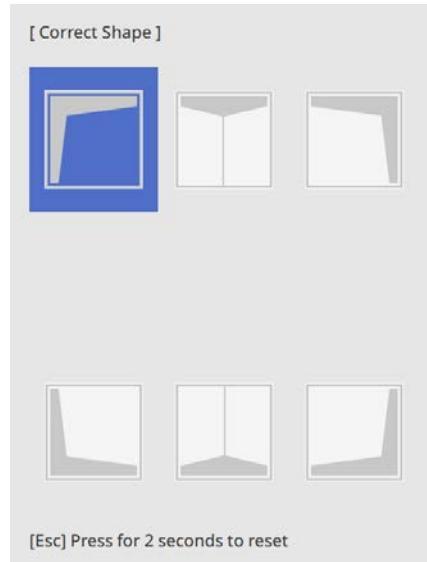
9 Press the arrow buttons to adjust the image shape of the selected area as necessary.
