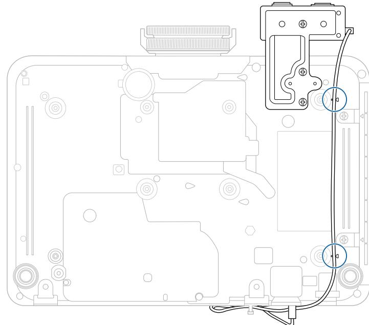
**2** After connecting the end of the USB cable to the projector, loop the cable tie through the cable holder of the projector, and then fold the USB cable and fix with the cable tie.
