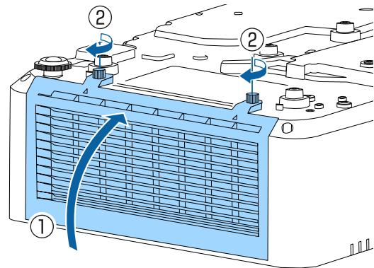
**3** Loosen the screws and open the air filter cover.
