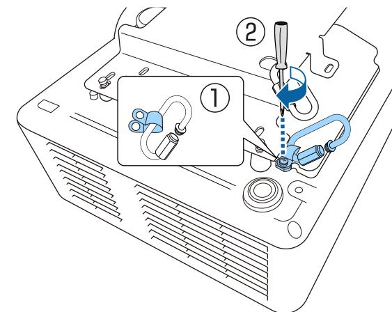
**3** Loop the safety wire through the carabiner on the ceiling mount, and attach both ends to the carabiner on the projector.
