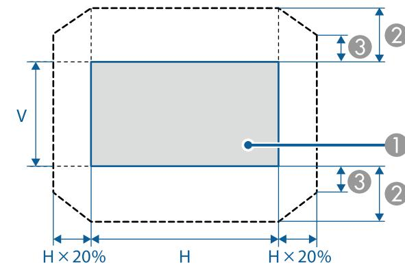
① Projected image at the center of the lens shift adjustment range
