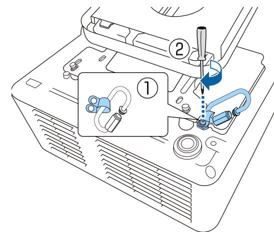
**2** Loop the safety wire through the hole in the ceiling mount, and then attach both ends to the carabiner.
