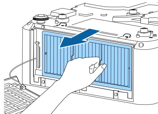
**6** Tap each side of the air filter 4 to 5 times to shake off any excess dust.
